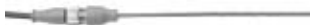
Part No. 3165-Lxx DIN A ML probe, -200°C..500°C, stainless steel, bendable, LS = 350 mm, D = 3 mm
